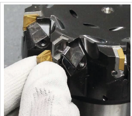
Fig. 8: Removing the indexable insert
