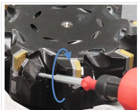
Fig. 14: Tightening the clamping jaw
