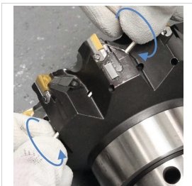
Fig. 6: Loosening the clamping jaw
